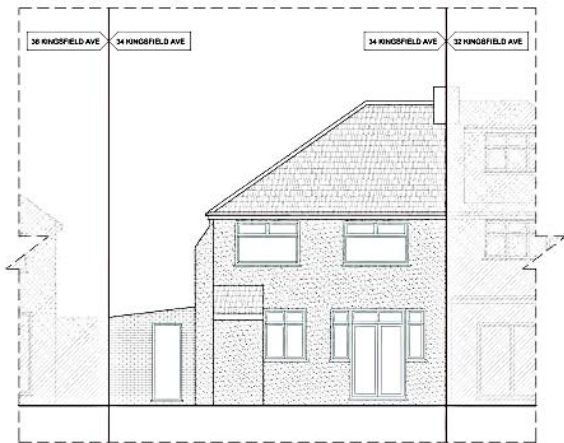
2 EXISTING REAR ELEVATION
